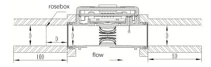
5.3.3 For ventilators and other compact space occasions, the structure of the airway at the inlet end can be adjusted as shown in the diagram to adjust the airflow distribution
