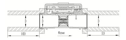
5.3.2 For occasions where the installation space is insufficient, rectification
